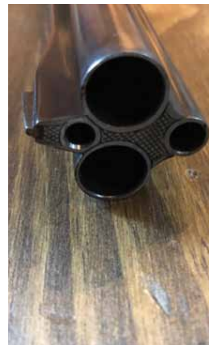
The muzzle end of a vierling, or four-barrel gun. This one has an 8x57R rifle barrel, a .22LR barrel, and two 16-gauge shotgun barrels.
