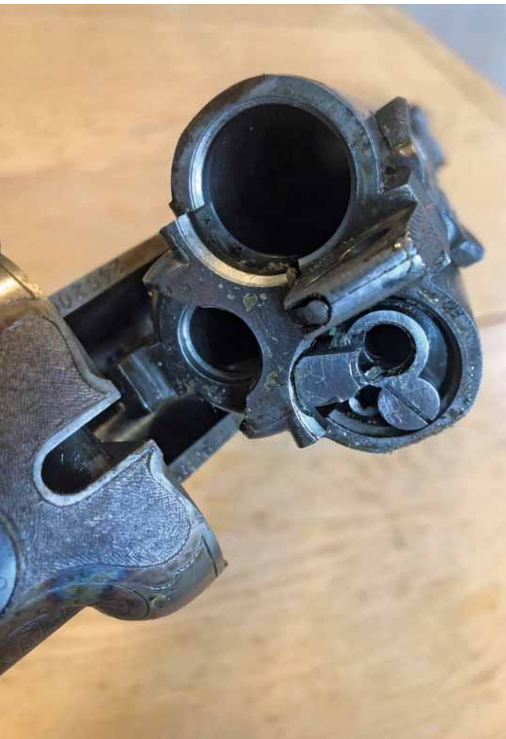
This is a Suhl drilling with a 7x57R rifle barrel and two 16-gauge barrels. An extra .22 rifle barrel has been installed inside the right shotgun barrel.
